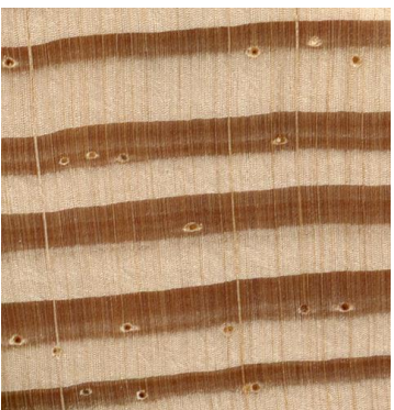
Figure 4: Longleaf Pine Endgrain (10X)
